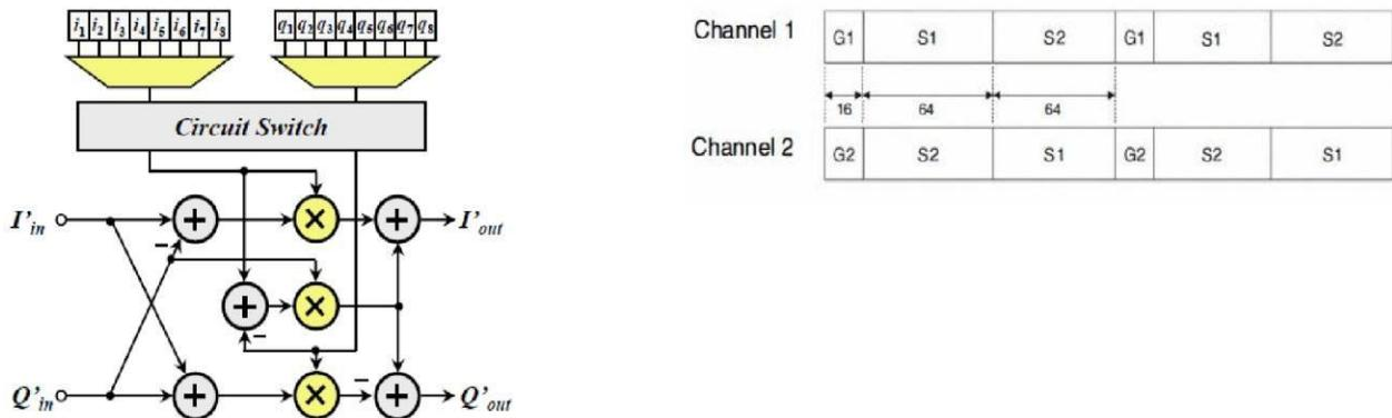
Figure 8: Complex Multiplier in Fig. 8, this circuit is responsible for the computation of multiplication by twiddle factor in Fig.7, which is also an important circuit of FFT/IFFT processor. The word length multiplier used in Fig.8 adopts a low-error fixed-width booth multiplier for hardware cost reduction.
