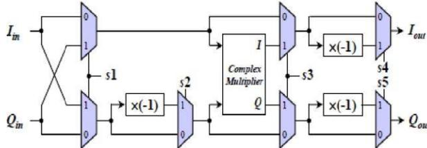
Figure 7: Reconfigurable Complex Constant Multiplier
