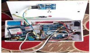
Fig. 7 Integrating GSM module with other devices to implement SMS notification
