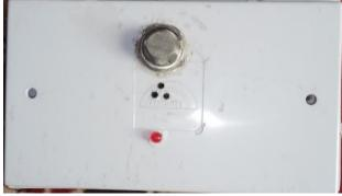
Fig. 12 Complete gas leakage detector device ready and encased in a parterres
