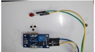
Fig. 8 Addition of MQ-5 gas sensor and LED indicator to the entire circuit
