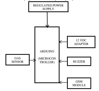
Fig. 4 Microcontroller System Architecture for smoke detection
