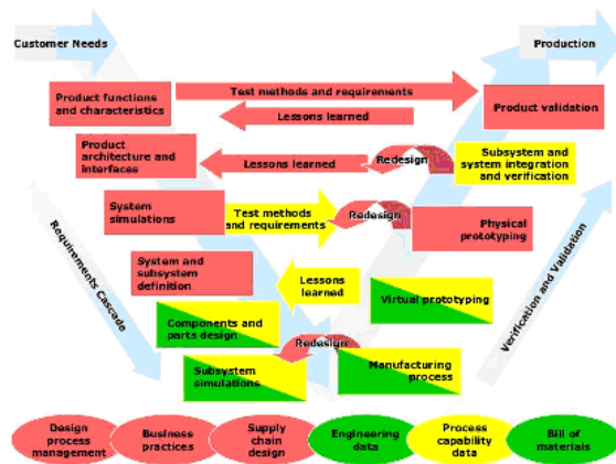
Figure 2: “V” Process Model modified to indicate the potential for a completely unified process approach [1]
