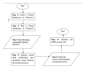
Figure 1. Architectural Diagram of performance measurement of Guest OS Virtual machine
